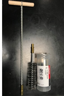
Figure 1 Typical drill and steel bristle brush for cleaning (left and center). Drilling with vacuum assistant (right).
